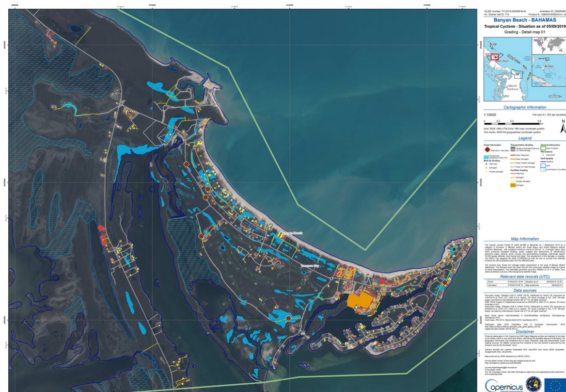
Figure 4-8: Example of a damage grade assessment map produced by CEMS after the hurricane “Dorian” hit the Bahamas in September 2019.
